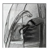
3. Select your spraying tip, insert screen filter and thread onto the 11/16 brass adaptor. Tips should be hand tightened only to provide a seal. Internal tip O Rings provide a "No Wrenches Required" seal. You can also connect directly to the Trigger Gun
