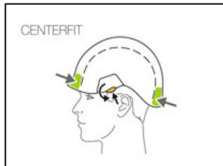
The CENTERFIT feature allows you to center the helmet on the head using the two side adjustment wheels.
