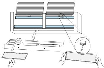
Removable tray holds our large (21-7/8" x 4-7/8") or standard (16-7/8" x 4-7/8") Glueboards for Touch-Free Maintenance. Additional (optional) glueboards may be inserted into the clips (behind top lamp) to increase total glue area.
