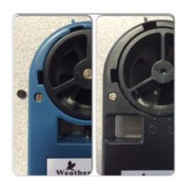
On the back side of the WeatherHawk wind meter there is a small screw located to the lower left of the impeller as seen in the pictures to the left. It may be covered by a small rubber cover.
